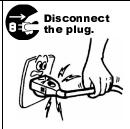
When unplugging the power cords, be sure to hold and pull on the plug portion. Pulling on the cord portion may cut or expose the internal wires and cause **fire** or **electric shock**.
